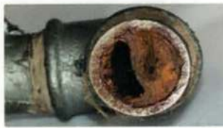
Pipe with scale deposits
